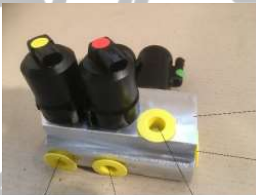
FB1: pressure line to left strut FB2: pressure line to right strut SP: pressure line to big accumulator T: return line P: pressure line from pump
